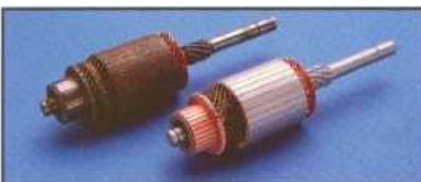
Armature cleaned with glass beads
