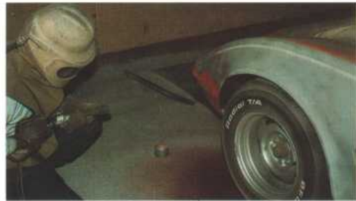
Rapid paint removal, with gel coat and body filler preserved.
