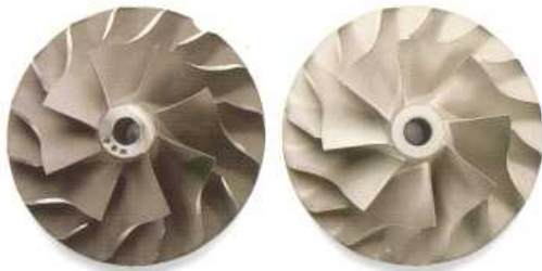
Finishing and removal of loose burrs on compressor wheels
